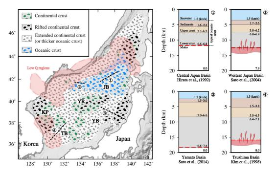
**Figure 4.** Crustal structures of the Japan Sea back-arc (modified from Tamaki et al. (1992)). Different crust types are indicated by green, black, gray, and blue spots. The red-shaded areas indicate strongly attenuated regions. The black-dashed lines marked with serial numbers represent previous seismic survey lines (Hirata et al., 1992; H. Kim et al., 1998; Sato et al., 2004, 2014), with their layered structures shown on the right.
