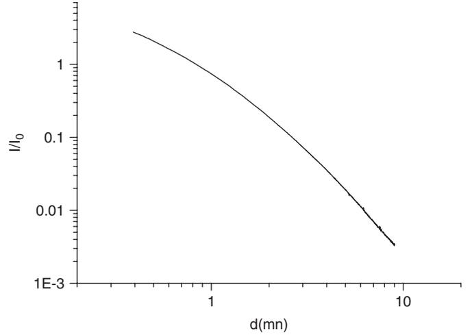
Fig. 2. Experiment curve. The material of the attenuation is Al.
