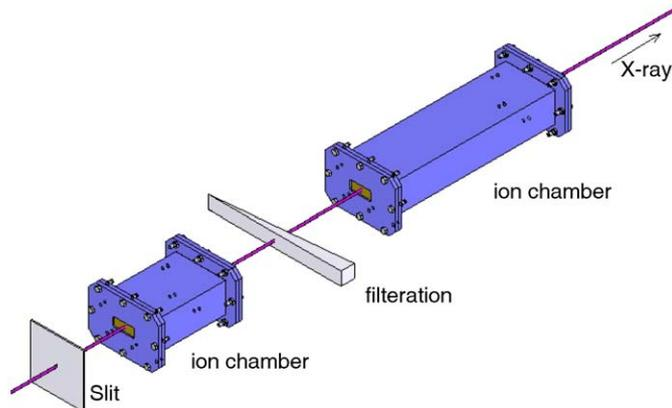
Fig. 1. Outline of the experimental setup. The slit was used to limit the incident X-ray to 0.1 mm ( $H$ )  $\times$  1 mm ( $V$ ).
