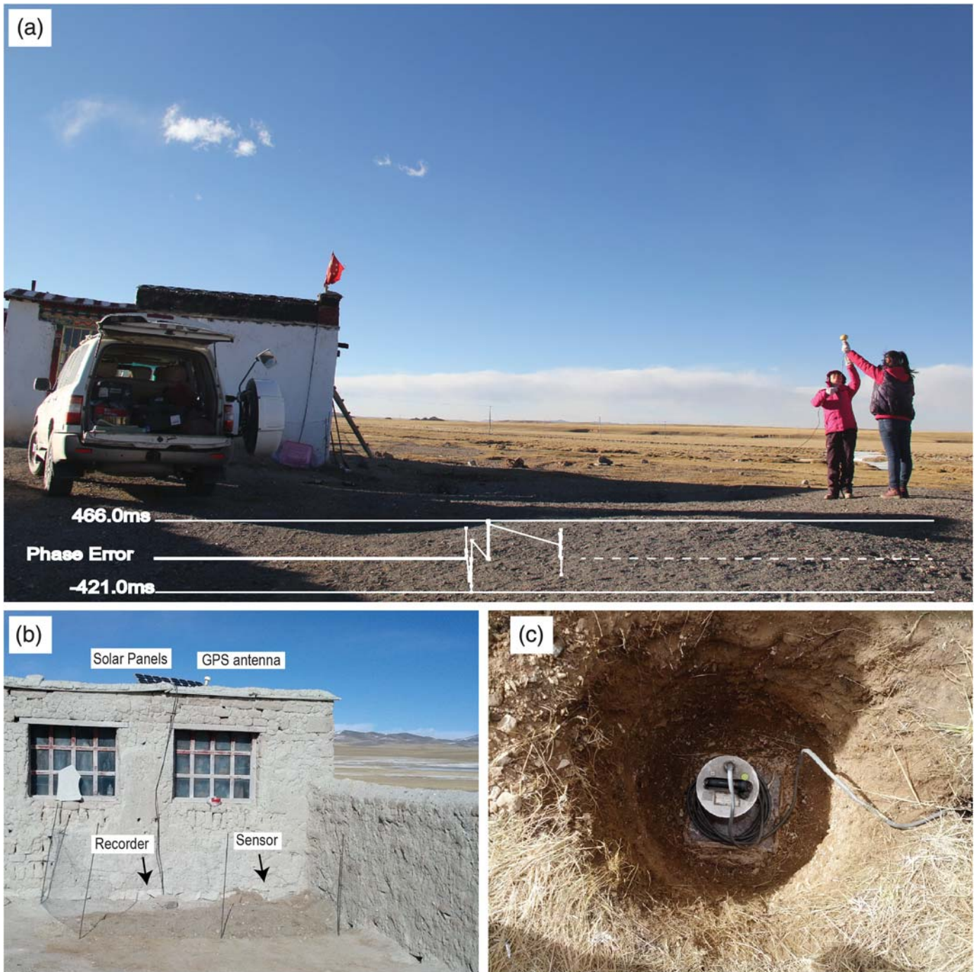
▲ Figure 2. Field deployment of a station. (a) Overlook of station QANM, located at the northeastern corner of a Tibetan house, when we were testing a Global Positioning System (GPS) antenna because of the bad status of health for its GPS clock, shown by the overlain phase error curve at the bottom of (a), in which the dashed line means no GPS phase information. (b) Setup details for a station (WQAM), including solar panels, GPS antenna, and buried sensor and recorder. (c) Deployment of a sensor in the field. The sensor is seated on a granite pad fixed by plaster at the bottom of a 1-m-depth vault.
