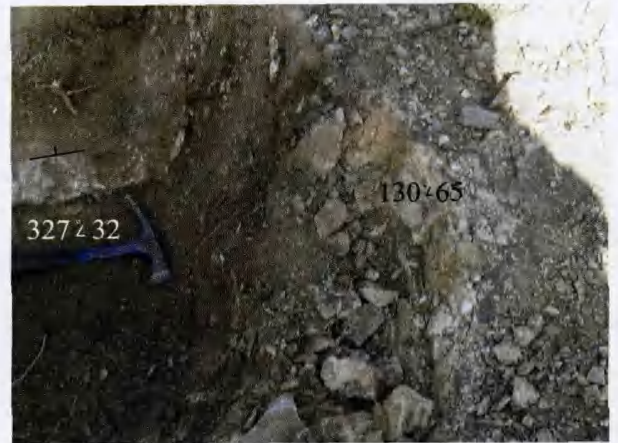
图3 霏细斑岩脉与砂岩的侵入接触关系 Fig. 3 Intrusion-contact relation of felsophyre vein with sandstone
